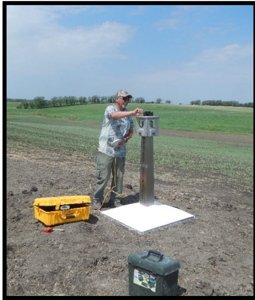
Surveying the position of a new Boundary Monument 795A.
