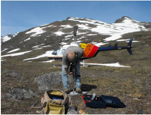
Establishing control point "Schepp" in British Columbia
