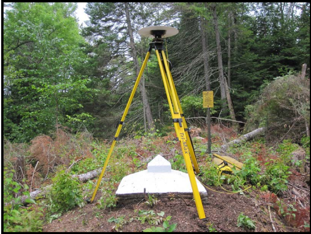
KWB-12-01: GPS control station set up on RM S-151 (Maine – Quebec)
