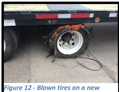
Figure 12 - Blown tires on a new Winston trailer (MT)
