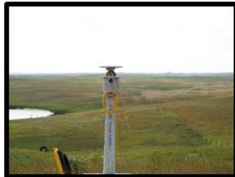
Figure 10 - GPS setup at Mon 584 during a control survey (ND/SK)
